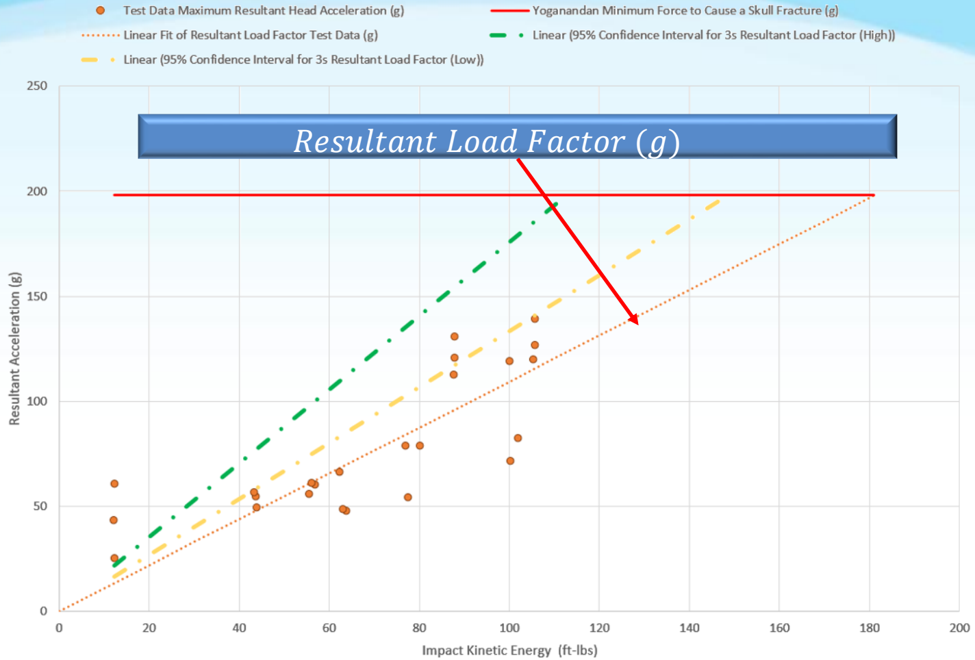
Figure 21 - Analysis of Resultant Impact for Skull Fractures versus Impact KE
